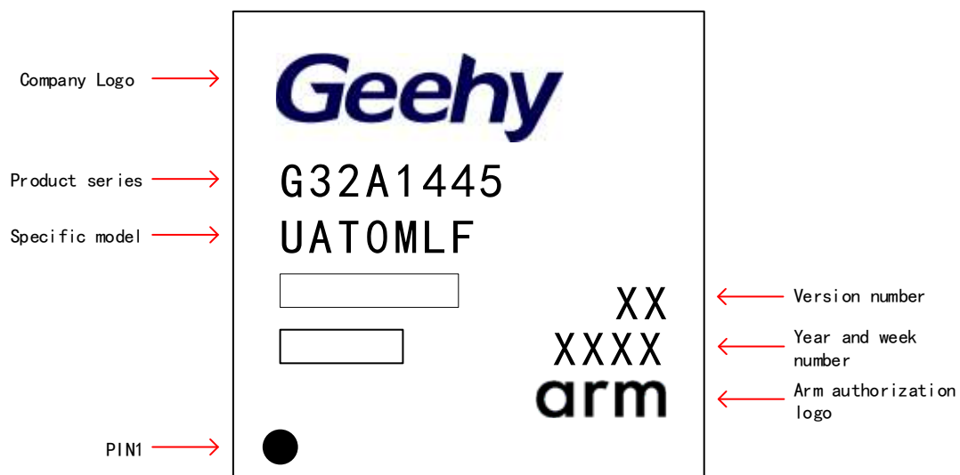
Figure 32 LQFP64 - 64 Pins, 7 x 7mm Diagram
